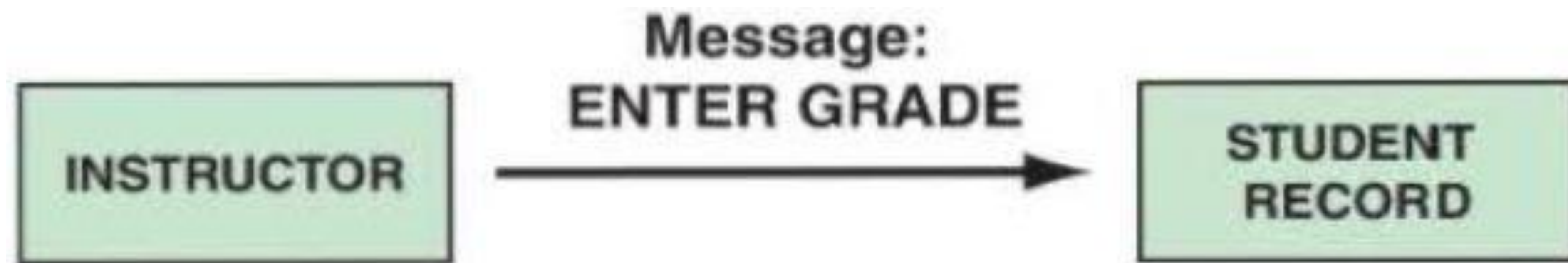
FIGURE 6-5 In a school information system, an INSTRUCTOR object sends an ENTER GRADE message to an instance of the STUDENT RECORD class.
